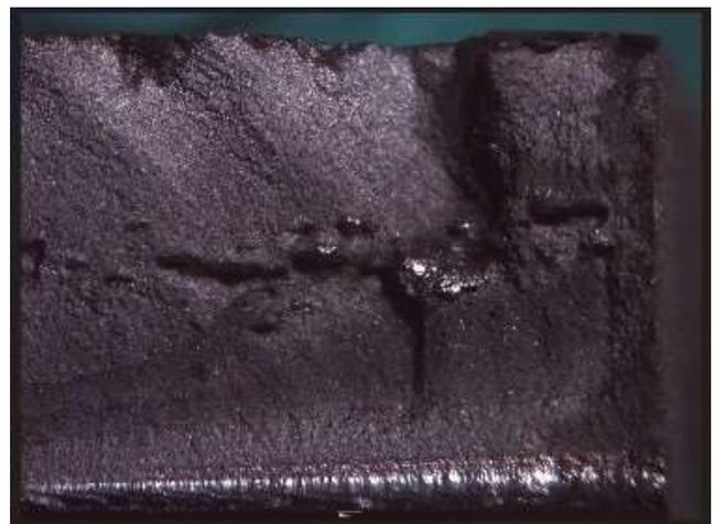
Figure 1. Front view of the fracture and crack growth in the specimen of interest
